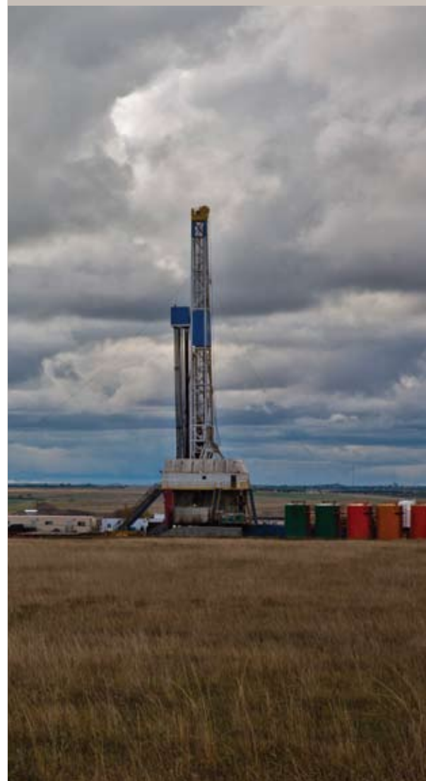
Above: Drilling rig for fracking operations in the Bakken shale formation (ND). ©David Gaylor/ Dreamstime.com
